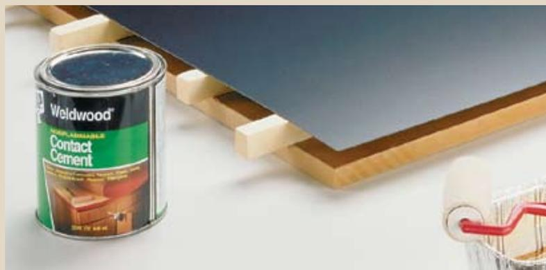
**JOINING THE PIECES.** The contact cement has to be almost dry before joining the two pieces. You can check it by simply dabbing it with your finger. It should look dull and feel slightly tacky, but shouldn't stick to your finger.
